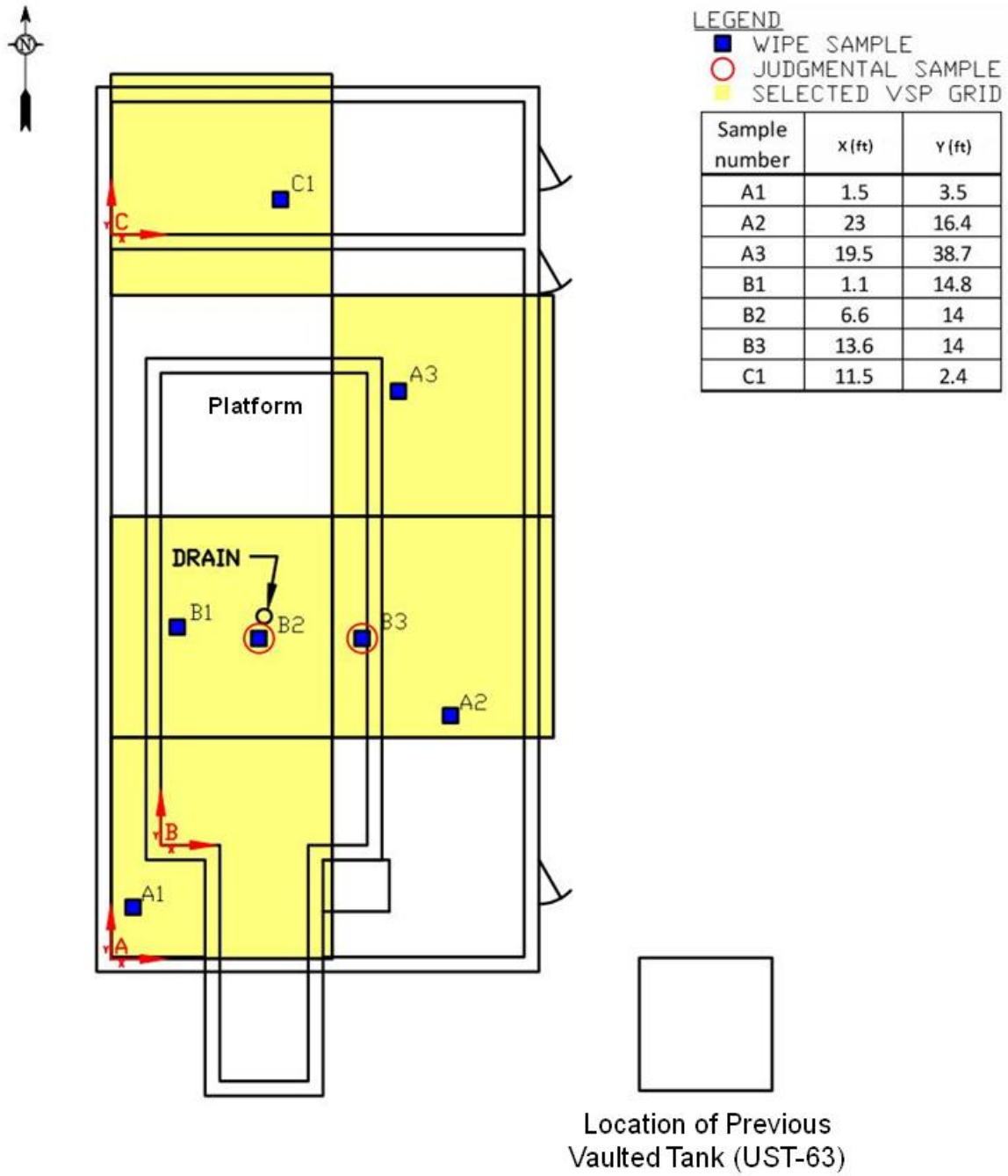
Figure 24. Sampling Locations for Building 27, Battery Shop
