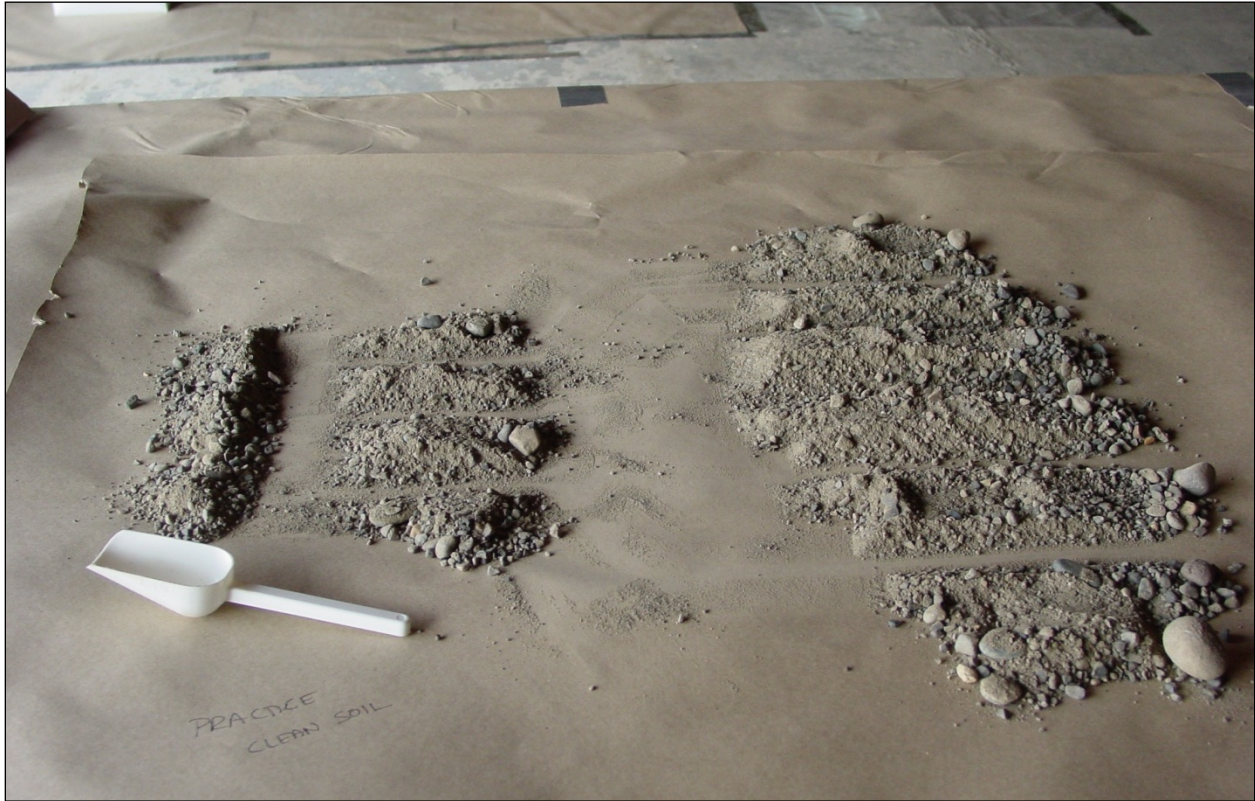
Figure 53. An Example of Incremental Sub-sampling
